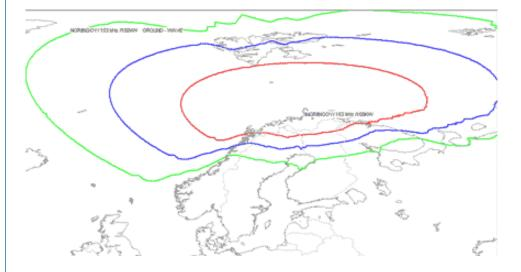
The illustration shows the coverage area of the Ingøy transmitter
