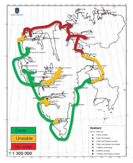
*The plan shows the results of the surveys* of the VSAT system 9-16th August 2010. Inmarsat C was also surveyed. Some places where VSAT was unstable (yellow) as is Inmarsat coverage due to other frequencies and antenna.
